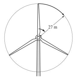
Show that the speed of the tip of this blade, with length  $27\,\mathrm{m}$ , is  $14.1\,\mathrm{m/s}$ , correct to 3 significant figures.
