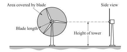
Wind turbines with longer blades generate more electrical power than wind turbines with shorter blades. Power is measured in kilowatts (kW).
